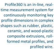
Profile360 employs CrossCheck laser line sensors manufactured by Bytewise to acquire thousands of data points around the profile and match them with a CAD template where key measurement parameters such as width, thickness, radius, and angle are extracted. Measurement parameters are compared to allowable control limits and displayed on the operator's terminal.
